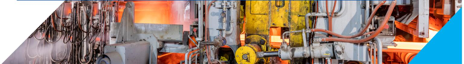
Big River Steel's caster plays a vital role in the abilities of our Flex Mill™. Slab thicknesses ranging from 2.170 to 3.350 are one of the attributes that allow our mill to “flex” between heavy and light gauges and meet the reduction ratios required to produce the most demanding steel grades.
